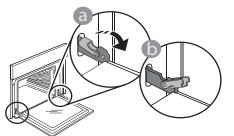
Simply remove the door by continuing to close it while pulling it upwards at the same time until it is released from its seating. Put the door to one side, resting it on a soft surface.
