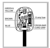
The wires in this mains lead are coloured in accordance with the following code: **BLUE "NEUTRAL"**
