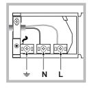
• Remove the wire clamp screw and the three contact screws L-N-+
