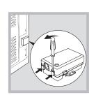
• Using a screwdriver, prise on the side tabs of the terminal board cover;
