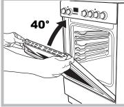
4.Press the two buttons on the upper profile and
