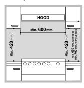
• If the cooker is installed underneath a wall cabinet, there must be a minimum distance of 420 mm between this cabinet and the top of the hob. This distance should be
