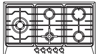
When the cookware diameter is smaller than 100mm, the user should use wok stand 2 putting it on the grate of the small (auxiliary) burner.
